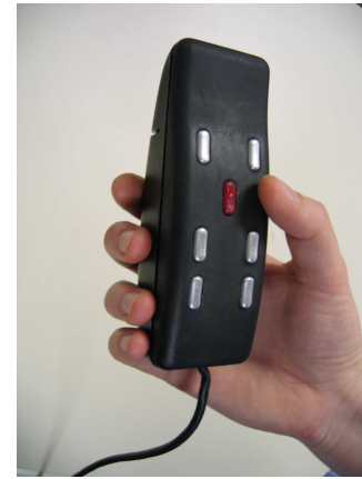
Figure 10: The modified Twiddler keypad used for input.
